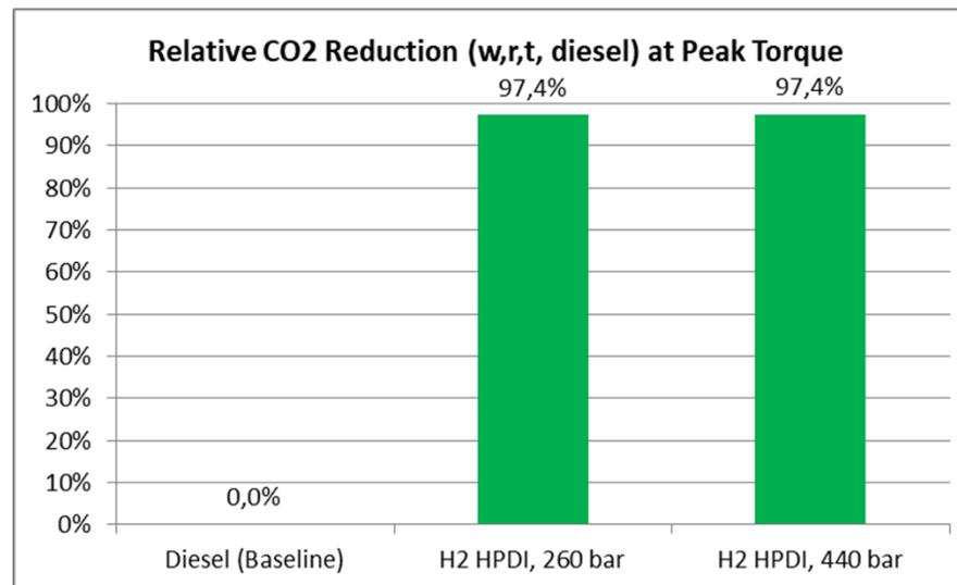
CO2 reduction of 97.4% from diesel baseline at the high load point with H2 HPDI
