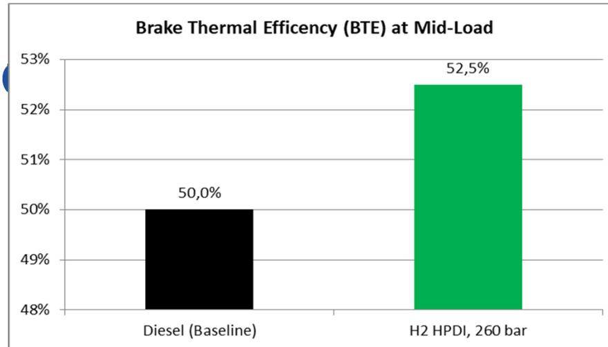
Over 50% brake thermal efficiency was predicted for H2 HPDI at the mid load point
