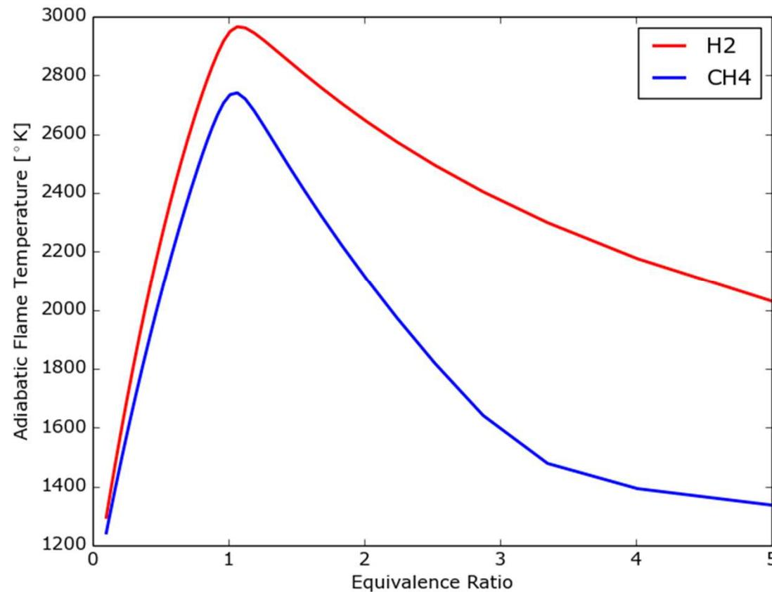
For methane on the fuel-rich side, the AFT decreases much faster compared to hydrogen. This is due to the fact that several reaction mechanisms such as the steam-methane reforming reaction and pyrolysis reactions are strongly endothermic.
