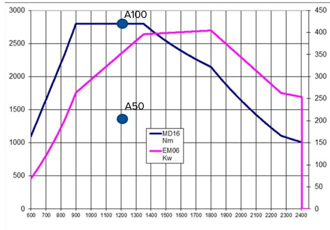
Torque Curve of Base Diesel Engine and Simulated Points
