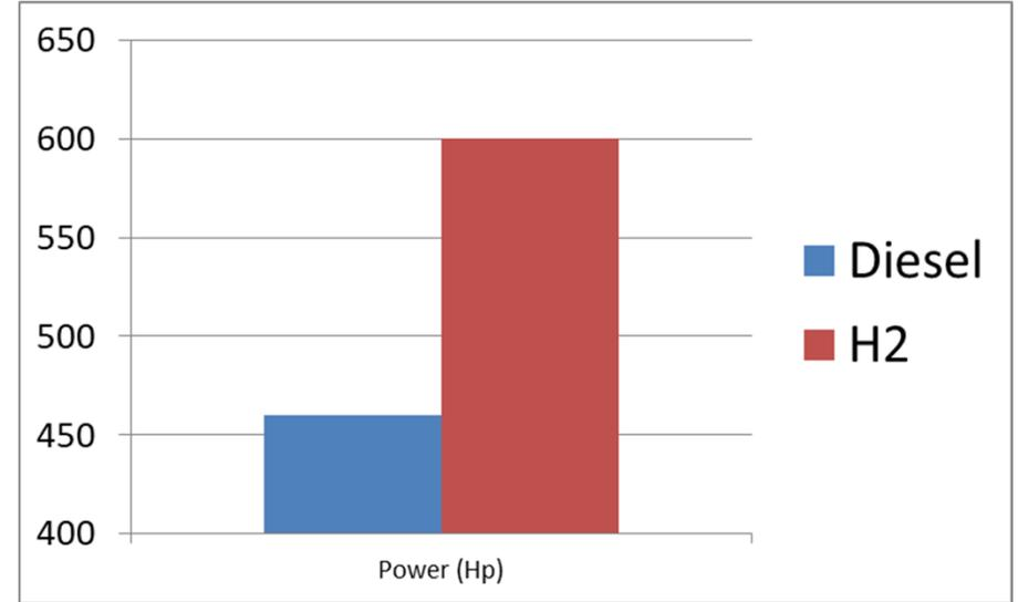
Torque and power comparison of 13-liter engine with diesel and with H<sub>2</sub> HPDI (engine limitations like PCP, exhaust temp, and boost pressure kept below limit)
